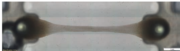
3D bioprinted human skeletal muscle cell tissue spanning between posts 1 day after printing. Source Novartis Basel.
