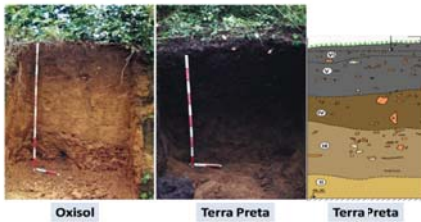
Fig. 13: soils in the Amazon Basin. left: a nutrient-poor soil, middle and right: Terra Preta de Indio with potsherds and a high content of charcoal (Glaser & Woods 2004).
