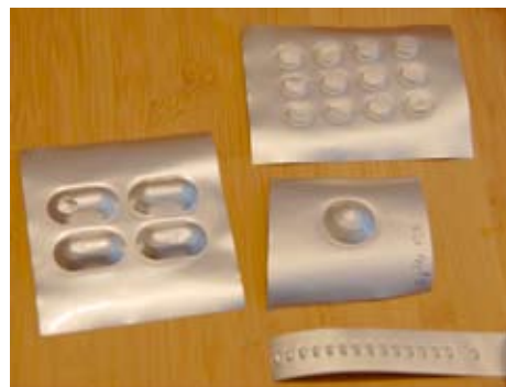
Fig. 1: Blisters formed by deep-drawing of a laminate.
