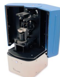
Fig. 1: From prototype to product: The PHELOS measuring instrument developed in the project for determining the angle-resolved radiation behaviour of OLEDs.
