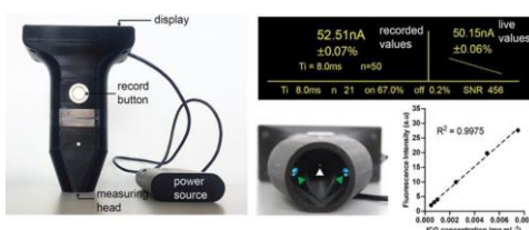
Fig. 1: Left: Autarkic hand tool with battery. Top right: Display. Middle: Measurement opening. Bottom right: Measured value versus actual marker concentration.
